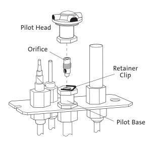
Figure 16. Pilot orifice removal and replacement.
